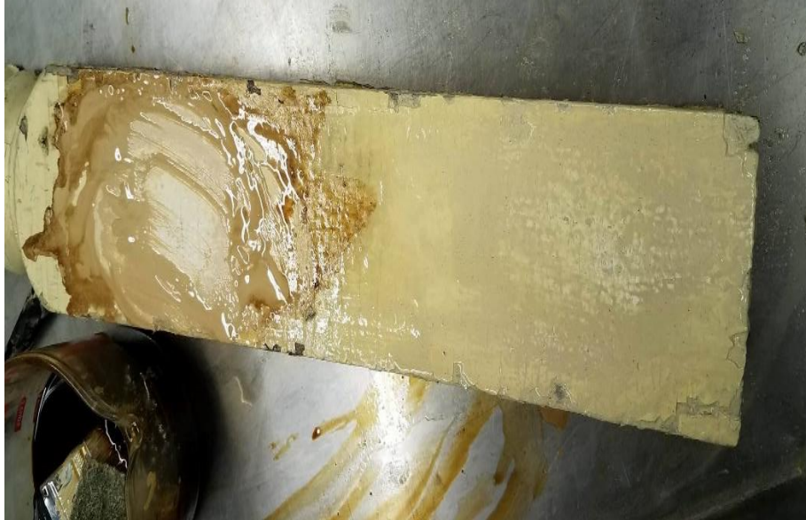
Figure 4: Testing results after 20 minutes (B7 on left side, Formulation #4 on right side)
