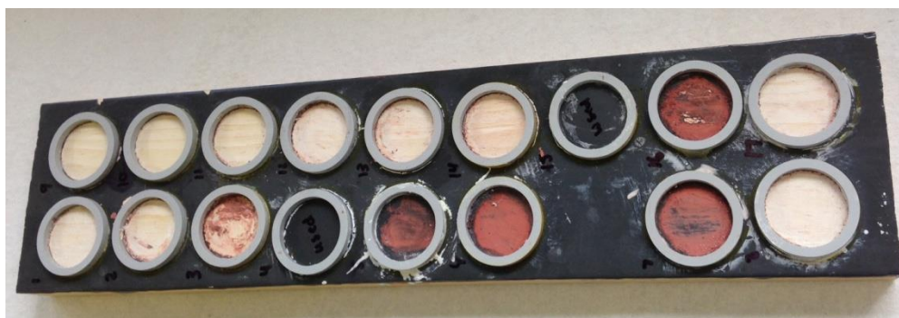
Figure 1: Wood coupon with ring gaskets after testing
